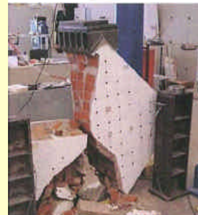
The crack of unreinforced masonry: the wall "bursts"
